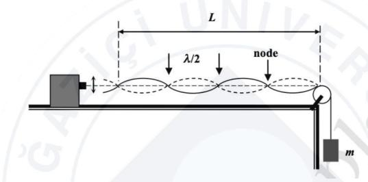
The wavelength of the waves travelling along the string with speed v depends on the tension **T** and mass per unit length of the string  $\mu$ . Tension is created by hanging mass **m**. Tension **T** is equal to **mg**.
