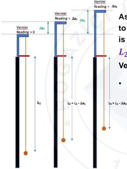
As the blue part that the string is attached to moves upward, the length of the string is shortened by the same amount. For  $L_2, L_3, L_4$  and  $L_5$ , you will only need the Vernier reading  $\Delta x$ .
