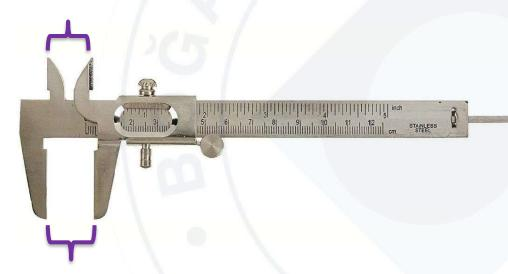
jaws for measuring outer dimensions \_\_\_\_\_
